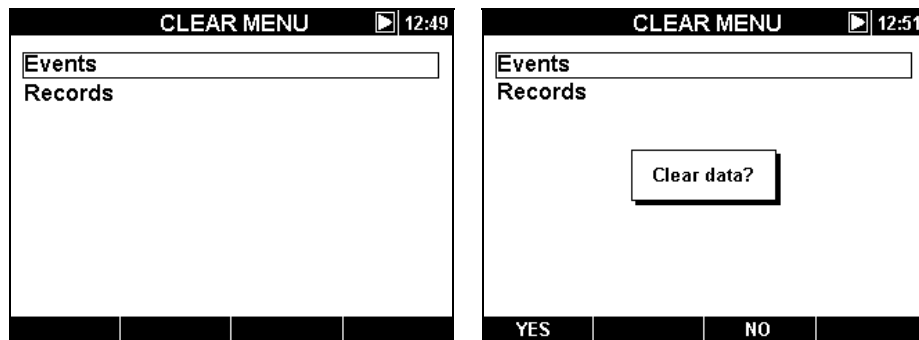
Figure 3.46: Clear memory menu and confirmation screen
